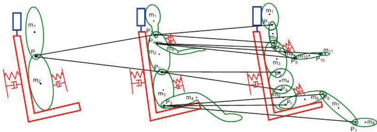
Fig. 1. The illustration of parameter identification of damping and stiffness with the use of 3 models of different complexity levels: a) a model with 3 degrees of freedom, b) a model with 7 degrees of freedom, c) a model with 13 degrees of freedom
