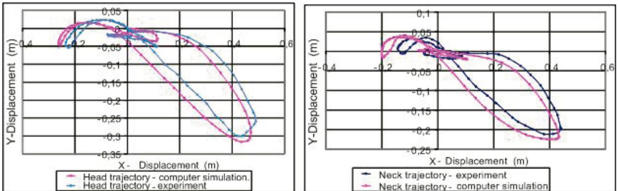
Fig. 3. The comparison of head and neck trajectories obtained in tests and computer simulation
