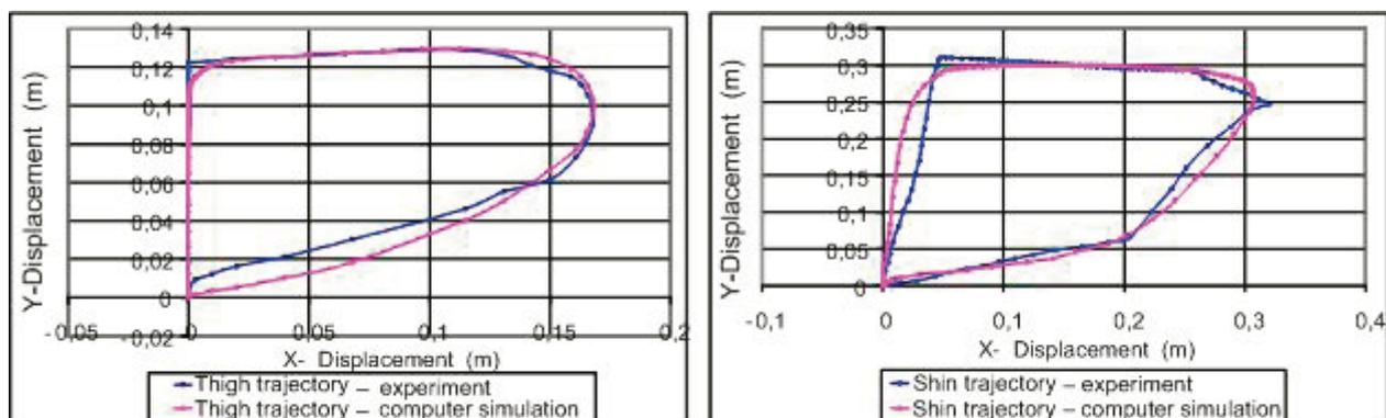
Fig. 6. The comparison of thigh and shin trajectories obtained in tests and computer simulation
