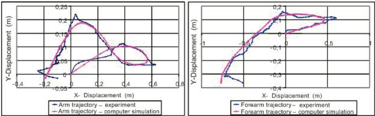
Fig. 7. The comparison of arm and forearm movement trajectory obtained in tests and computer simulation
