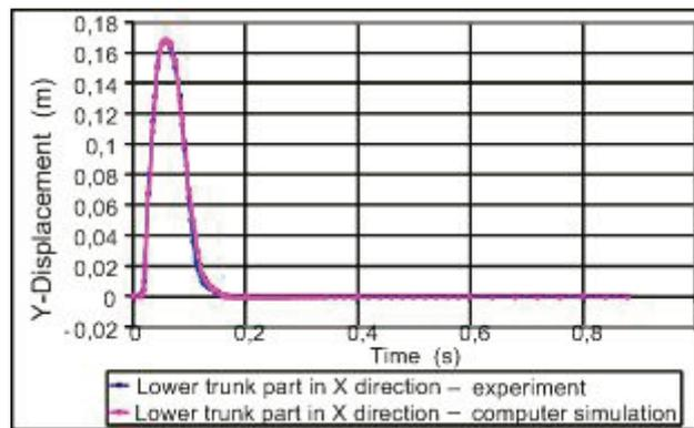
Fig. 5. The comparison of lower trunk part displacement obtained in tests and computer simulation
