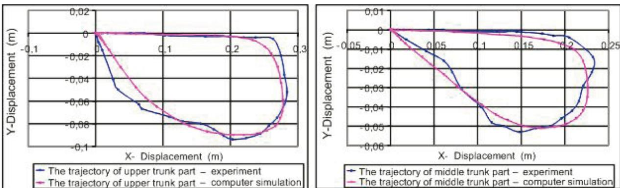
Fig. 4. The comparison of the movement trajectories of upper and middle trunk parts obtained in tests and computer simulation
