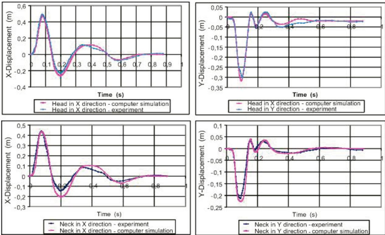
Fig. 2. The comparison of test results and the computer simulation of horizontal head and neck displacements
